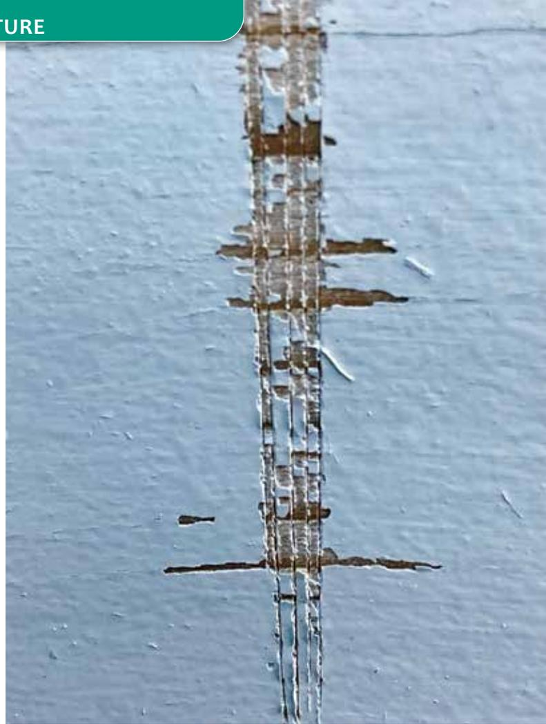
Test de quadrillage
